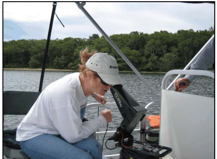
Wendy Gendron from ENSR looks through the viewing screen of the video camera system used to survey the distribution of freshwater mussels in Mystic Lake.
