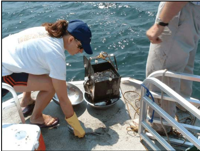
Kate Dunlap from ENSR prepares to remove a sample of "muck" from a full Eckman bottom dredge collected in Mystic Lake.
