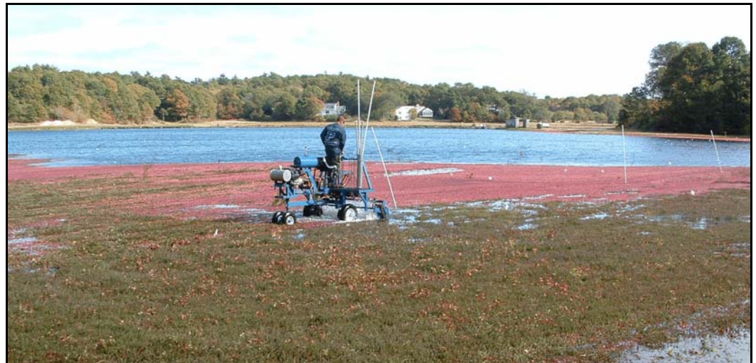
John Hamblin operating a water-reel cranberry harvesting machine in October 2008, with cranberries loosened from their vines floating in the flooded bog.
