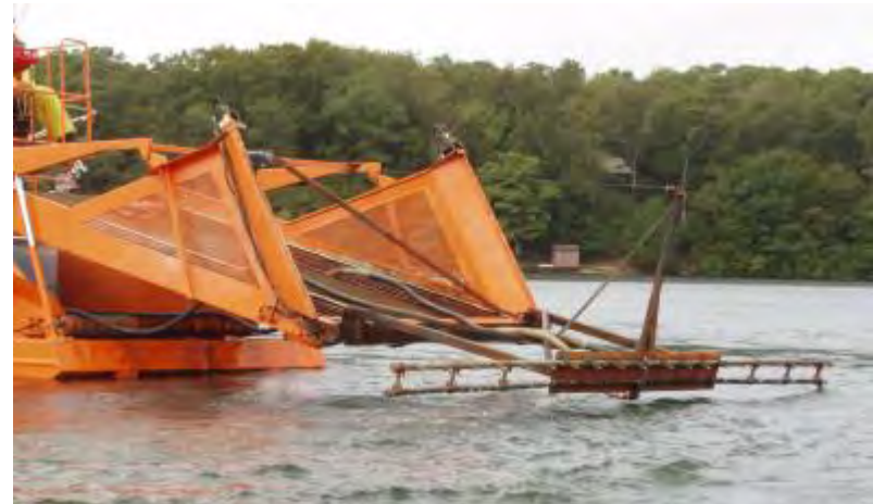
Manifolds before lowering to treatment depth.
