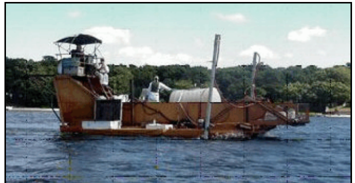
Motorized barge used for injecting alum solution into a lake.
